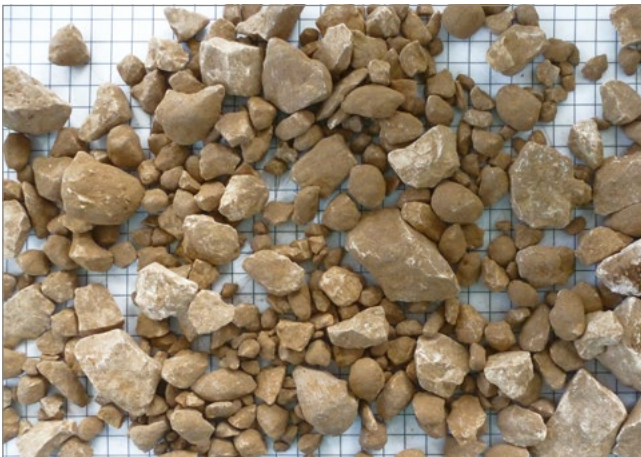
Screened products > 5 mm after Combimix mixing process
